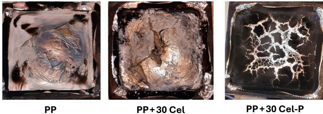
Figure 8. Images of char residues after MLC test of PP and cellulose-based composites.
